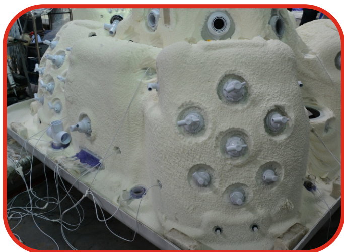
10mm High density insulation foaming on the spa shell
